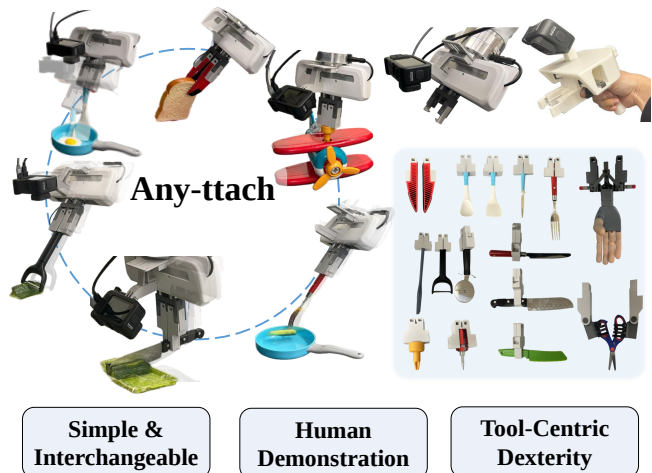
Fig. 1. Tool-centric design achieves dexterity and end-effector swapping with simplicity. Any-ttach enables robots to perform diverse manipulation skills by rapidly switching between interchangeable tool modules through a standardized mechanical interface. By externalizing task-specific contact geometry into tools, the system reformulates manipulation dexterity as tool selection and skill execution rather than complex end-effector control.
