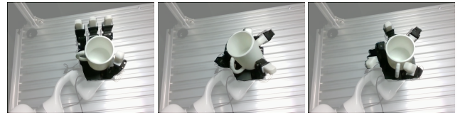
Fig. 8: Real-World Trajectory Replay. Simulated action sequences achieve consistent 90^\circ z-axis rotations when replayed in the real world.
