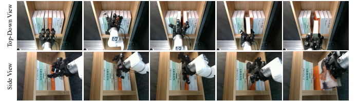
Fig. 7: Real-world Policy Execution. We show a temporal sequence (left to right) of the policy executing the shelf object singulation task.
