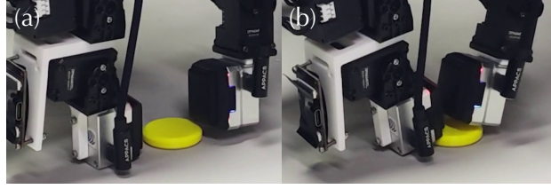
Fig. 9. GelSight failure in coin standing. The square sensor geometry makes edge wedging difficult in this setup.
