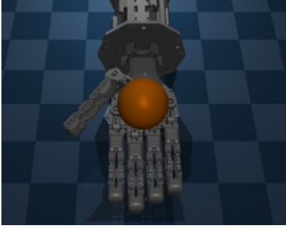
Fig. 10: CRAFT in MuJoCo Simulation. CRAFT grasping a sphere, with rolling contact joints modeled as equality constraints and joints treated as revolute constraints.
