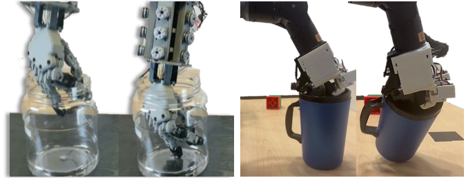
Fig. 13: Narrow Space Accessibility. CRAFT demonstrates the ability to fit into a narrow jar, while the bulkier Leap Hand V2 fails to enter the same workspace due to its rigid linkage size. Both cans have the same radius. Results reproduced with the help of the authors of Leap Hand V2 [24]; reproduced in two labs with different cans.
