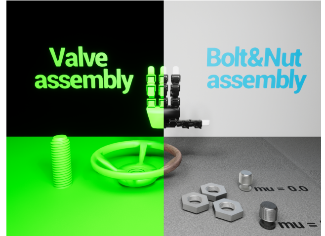
Fig. 1: Overview of ‘Leap hand assembly’ scenario consisting of four bolt–nut assembly tasks. The left half shows meshes used as colliders, while the right half shows meshes for rendering.
